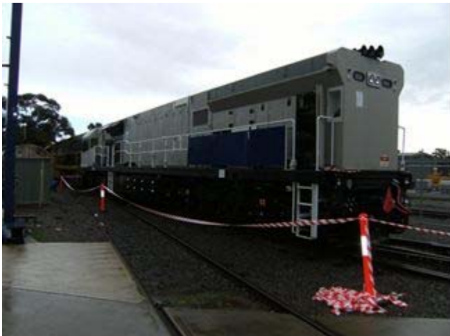
Photo 6 – 92 Class Locomotive During Load Testing
