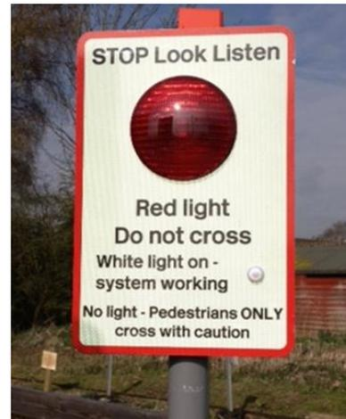
Figure 2: Warning lights for LCWS, Network Rail example
