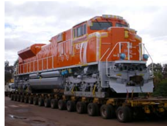
One of thirty new SD70ACe locomotives to move iron ore to Port Hedland. Photo: BHP Billiton
